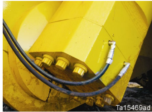
Spherical ball joint greased through cap – hole in ball is plugged
