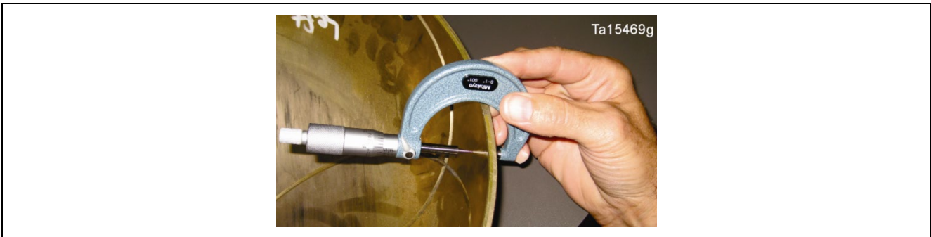
Figure 55. Measure liner thickness with a point micrometer
