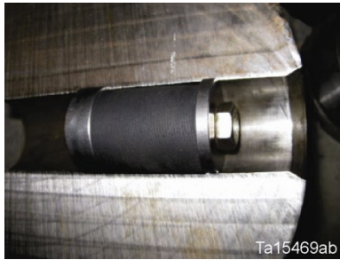
Spherical ball joint greased through cap – hole is plugged (refer to SIL 413)
