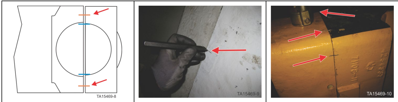
Figure 70. Align the cap sphere visually with the socket sphere and match mark with a chisel
