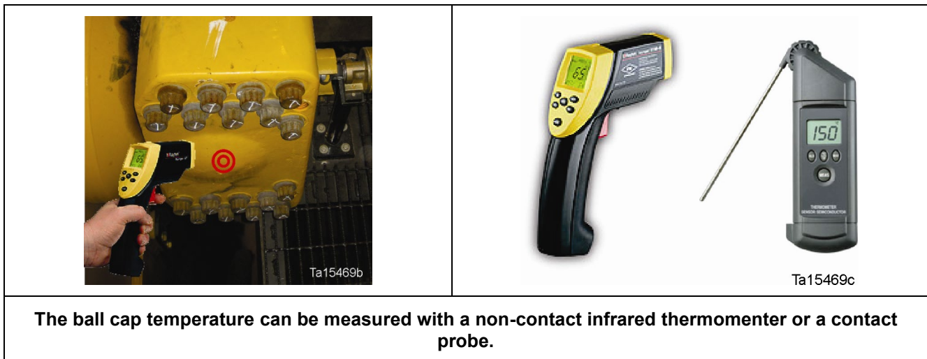
Figure 48. Measuring ball cap temperature
