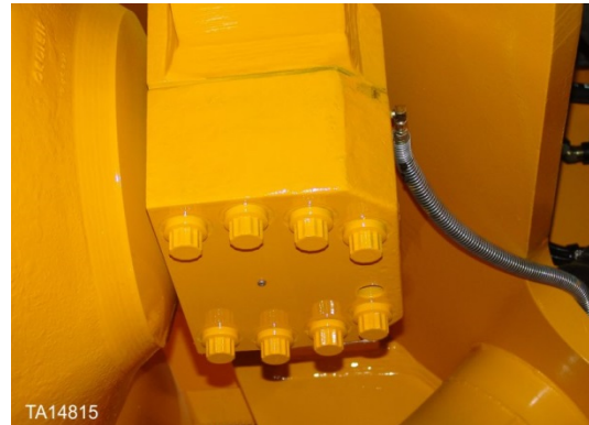
Figure 2. Rear axle - front ball cap shown - rear cap is the same
